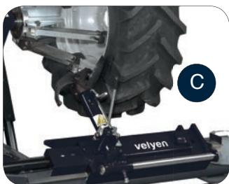
**(EN) TOOL-HOLDER ARM:** Tool-holder arm lifting and tool rotation are manually achieved through an on-purpose device. The special semi-spherical shape of the bead breaker disc allows to obtain a better penetration between rim and tyre bead in order to avoid damaging the wheel.
