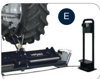
**(EN) CONTROL UNIT:** The machine is equipped with a low voltage portable control unit, easily movable inside the working area. The rational lay-out of control levers, buttons and pedals prevents the operator from making accidental and dangerous operational errors.
