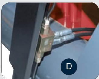
**(EN) SAFETY DEVICES:** The tyre changer has a number of safety devices designed to guarantee the utmost operator safety: check valves on self-centering chuck, hydraulic unit motor with overload cut-out system and safety lock device on tool holder arm.
